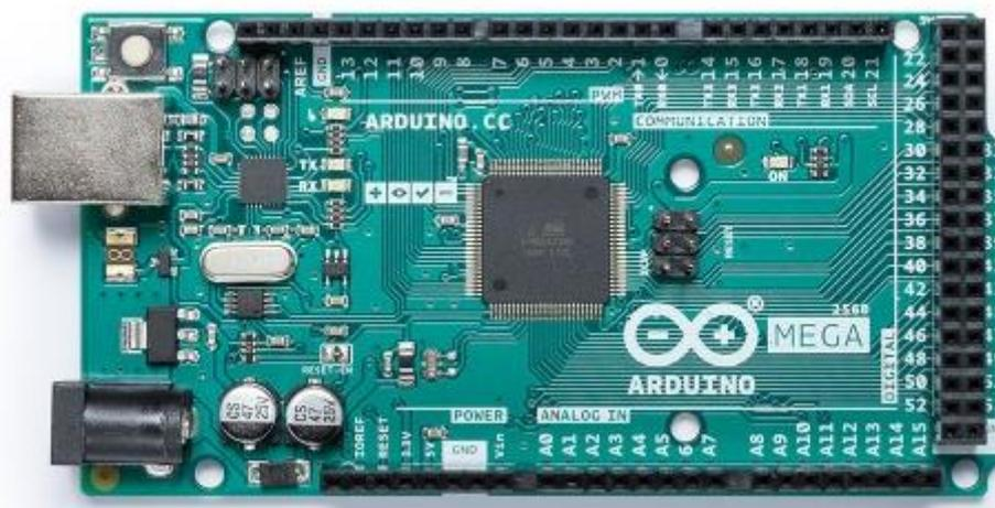
**Gambar 2.3 Arduino Mega 2560**
