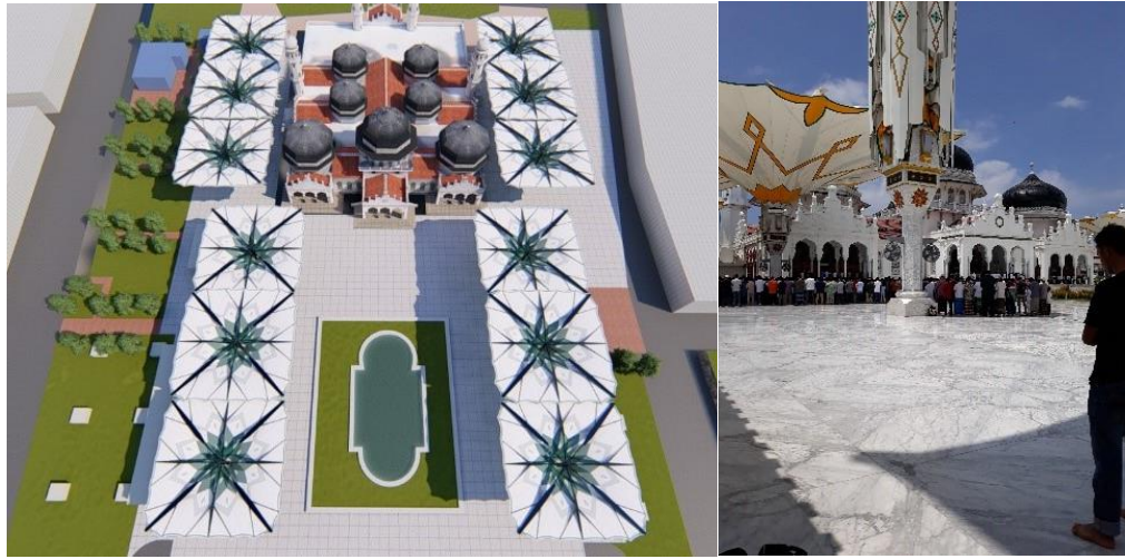
Figure 2. The positions of the umbrellas once all are open, and the large separations due to the limited shadings among the worshippers while conducting the prayer if the umbrellas are close
