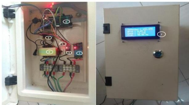
Gambar 8. Sistem *monitoring* portable Generator 3 fasa
