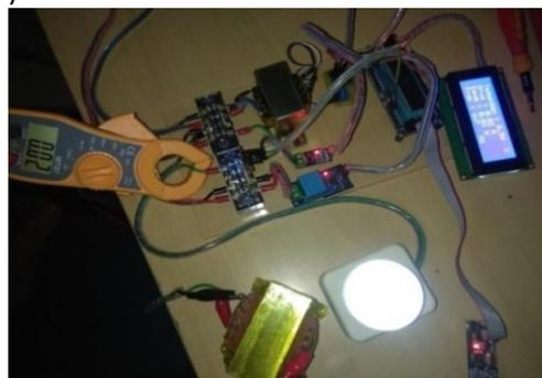
Gambar 10. Pengujian Sensor ZMPT201B
