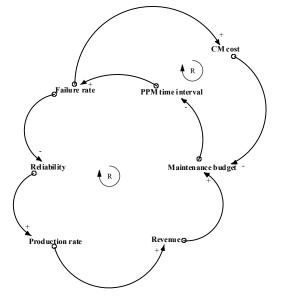
Figure 9. The Causal Loop Diagram (CLD)
