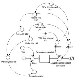
Figure 10. The Stock Flow Diagram (SFD)
