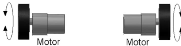
Figura 29: Mecanismo “Differential-drive”
