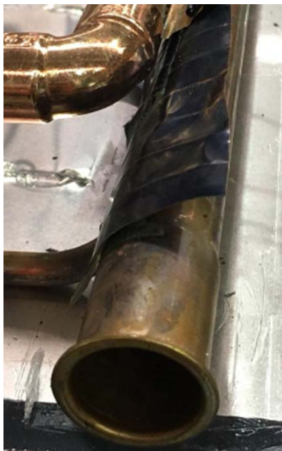
Fig.3: Placement of TEG between copper fins
