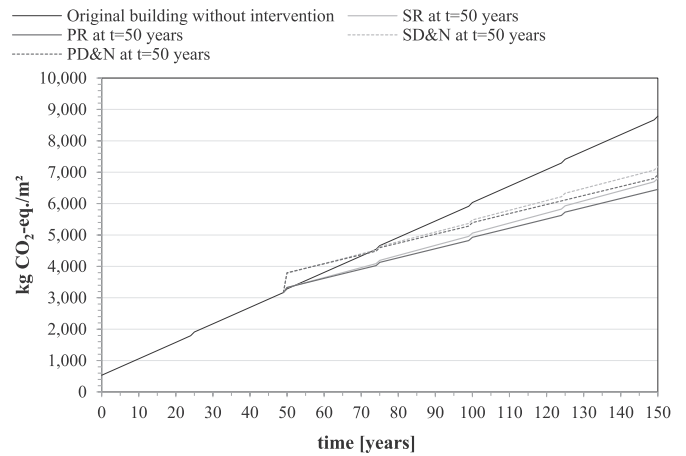
Fig. 1. kg CO 2 -eq./m 2 of the original building and different intervention alternatives at t = 50 years: SR, PR, SD&N and PD&N.
