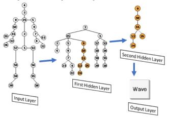
Fig. 6. Depiction of layers in classifier (on wave action)
