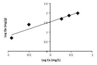
Fig. 15 Freundlich isotherm model for sorption of  $Cu^{2+}$  onto nZVMn
