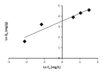
Fig. 19 Halsey isotherm model for sorption of Cu<sup>2+</sup> onto nZVMn
