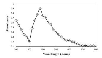
Fig. 1 UV-VIS spectrum of nZVMn
