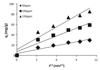
Fig. 11 Intraparticle diffusion plot for sorption of Cu<sup>2+</sup> onto nZVMn
