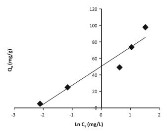
Fig. 17 Temkin isotherm model for sorption of Cu<sup>2+</sup> onto nZVMn
