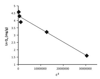
Fig. 18 DKR isotherm model for sorption of Cu<sup>2+</sup> onto nZVMn
