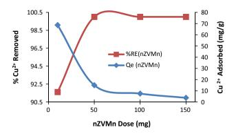
**Fig. 4** Effect of nZVMn dose on  $Cu^{2+}$  adsorbed by nZVMn. Experimental conditions: optimum  $Cu^{2+}$  concentration = 100 ppm; volume of  $Cu^{2+}$  solution = 50 mL; pH = 5, stirring speed = 200 rpm, contact time = 60 min, and temperature =  $25 \pm 2$  °C
