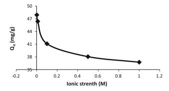
**Fig. 24** Ionic strength on  $Cu^{2+}$  adsorbed onto nZVMn. Experimental conditions:  $Cu^{2+}$  concentration = 100 ppm; volume of  $Cu^{2+}$  solution = 50 mL; nZVMn dose = 100 mg; pH = 5, contact time = 60 min, stirring speed = 200 rpm and temperature = 25  $\pm$  2 °C
