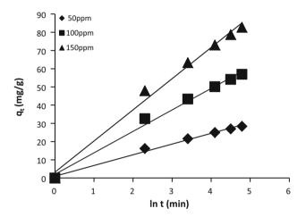
Fig. 9 Elovich kinetics model plot for sorption of Cu<sup>2+</sup> nZVMn
