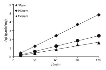
Fig. 8 Pseudo second-order kinetics plot for sorption of  $\mbox{Cu}^{2+}$  onto nZVMn
