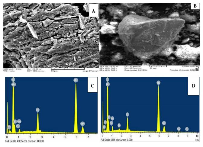
Fig. 12 (a) SEM image of nZVMn before sorption (b) SEM image of nZVMn after sorption (c) EDXspectrum of nZVMn before sorption, (d) EDX spectrum of Cu(II) loaded nZVMn after sorption
