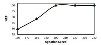
**Fig. 5** Effect of agitation speed on  $Cu^{2+}$  adsorbed onto nZVMn. Experimental conditions: optimum  $Cu^{2+}$  concentration = 100 ppm; volume of  $Cu^{2+}$  solution = 50 mL; nZVMn dose = 100 mg; pH = 5, contact time = 60 min, and temperature = 25  $\pm$  2 °C
