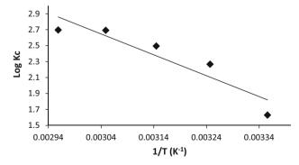
Fig. 23 Van't Hoff plot on sorption of Cu<sup>2+</sup> onto nZVMn nano-adsorbent
