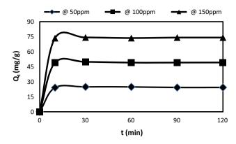
**Fig. 6** Effect of contact time on  $Cu^{2+}$  adsorbed onto nZVMn. Experimental conditions:  $Cu^{2+}$  concentration = 100 ppm; volume of  $Cu^{2+}$  solution = 50 mL; nZVMn dose = 100 mg; pH = 5, stirring speed = 200 rpm, and temperature =  $25 \pm 2$  °C
