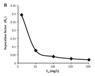
Fig. 16 a Langmuir isotherm model for sorption of  $Cu^{2+}$  onto nZVMn, b separation factor on sorption of  $Cu^{2+}$  onto nZVM
