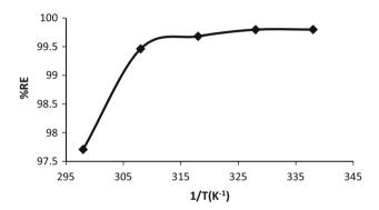
**Fig. 22** Effect of temperature on  $Cu^{2+}$  adsorbed onto nZVMn. Experimental conditions: optimum  $Cu^{2+}$  concentration = 100 ppm; volume of  $Cu^{2+}$  solution = 50 mL; nZVMn dose = 100 mg; pH = 5, contact time = 60 min, and temperature = 25  $\pm$  2 °C
