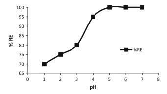
**Fig. 13** Effect of pH on  $Cu^{2+}$  adsorbed onto nZVMn. Experimental conditions: optimum  $Cu^{2+}$  concentration = 100 ppm; volume of  $Cu^{2+}$  solution = 50 mL; nZVMn dose = 100 mg; stirring speed = 200 rpm, contact time = 60 min
