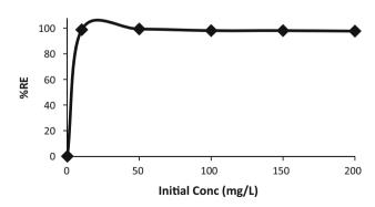
**Fig. 14** Effect of initial concentration on  $\text{Cu}^{2+}$  adsorbed onto nZVMn. Experimental conditions: optimum  $\text{Cu}^{2+}$  concentration = 100 ppm; volume of  $\text{Cu}^{2+}$  solution = 50 mL; nZVMn dose = 100 mg; pH = 5, contact time = 60 min, and temperature = 25  $\pm$  2 °C
