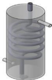
**Gambar 17. Kondensor Spiral Tipe Vertikal**
