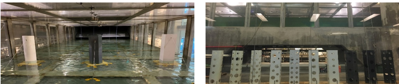
Fig. 4. View from inside the SUSTAIN tank (left) and SEAHIVE units ready for testing (right).
