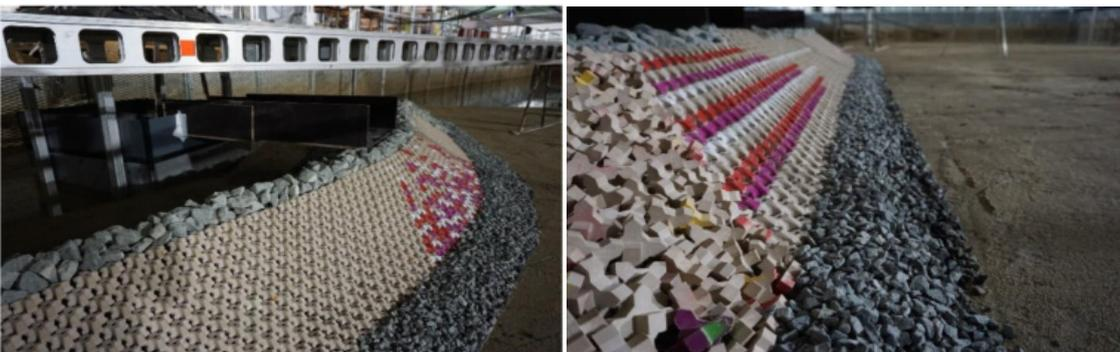
Fig. 8. Breakwater model in 3D tests, Curved section and XblocPlus / Xbloc Interface
