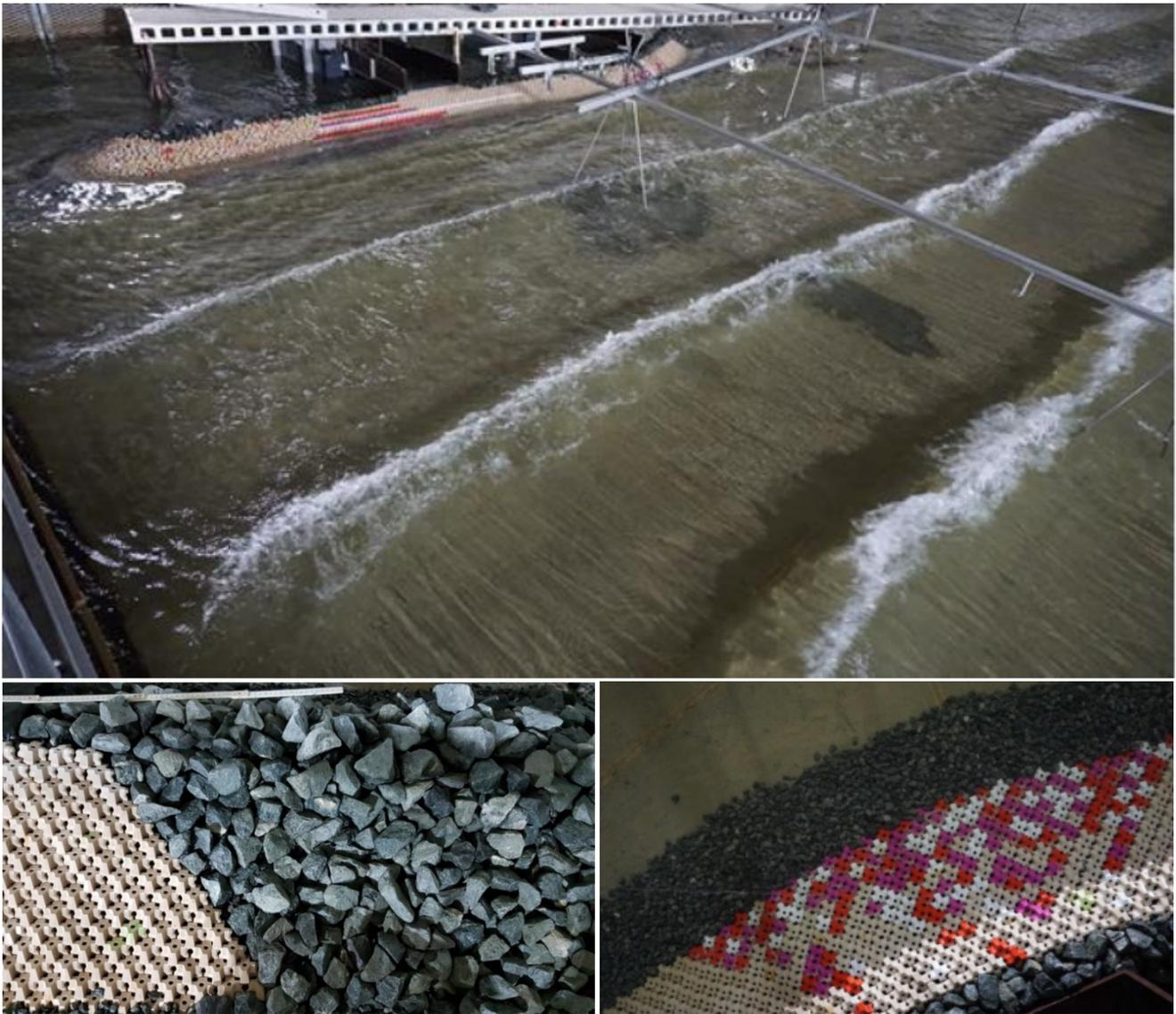
Fig. 10. Breakwater model in 3D tests, XblocPlus / Rock Interface and Curved section
