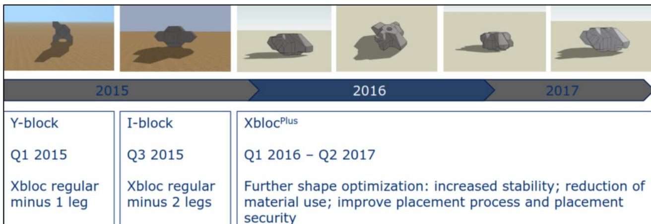
Fig. 3. XblocPlus Armour unit shape development timeline
