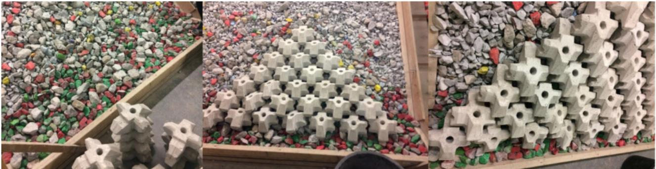
Fig. 13. Placement of XblocPlus units on an under layer significantly exceeding construction tolerances
