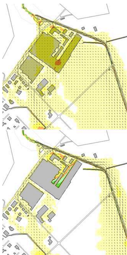
Fig. 10: Complex modelled as impermeable obstacle, Strickler 0 \text{ m}^{1/3}/\text{s} (above) and as permeable, Strickler 1 \text{ m}^{1/3}/\text{s} (below) (Background: [5])
