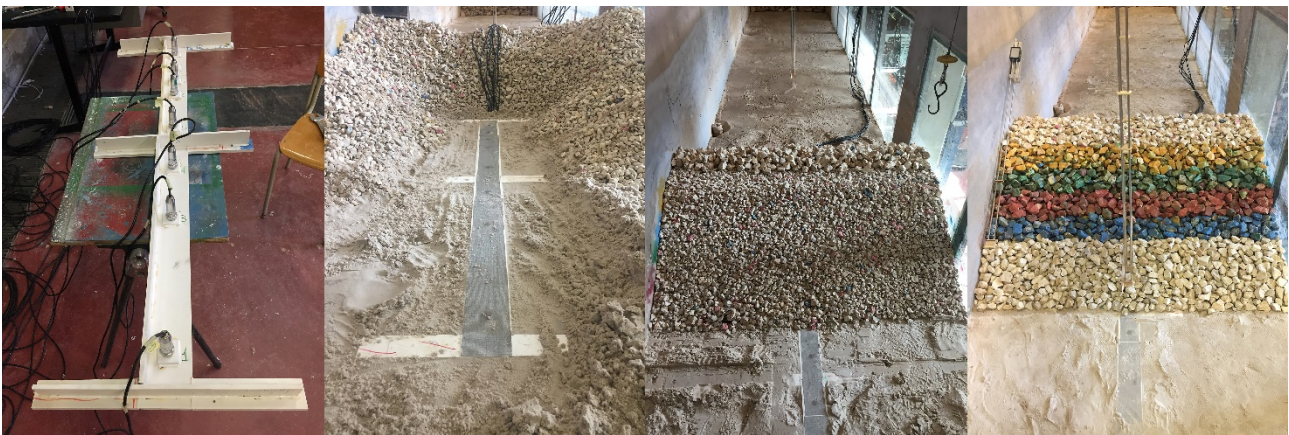
Fig. 2. Layout of pressure gauges deployed in the wave flume.
