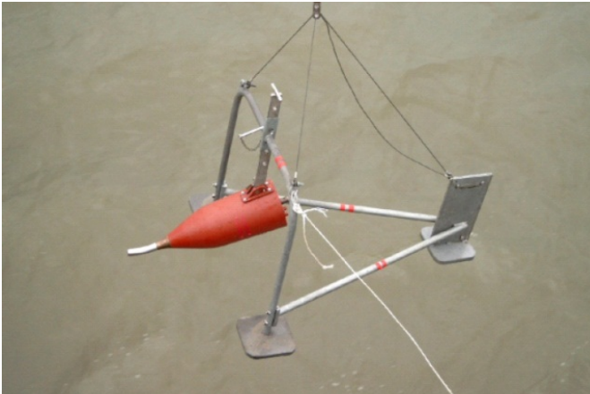
Figure 3 – Delft bottle on frame to measure sand transport just above the bottom.
