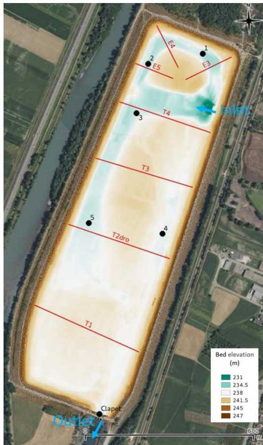
Figure 3: Location of ADCP cross-sections (red lines) and sediment concentration measurements (black points).
