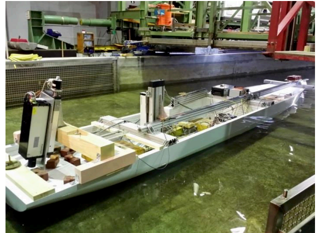
Figure 2. A 1D and a 2D-LDV mounted on the model of a 14000 TEU Containership to detect the near wall flow conditions. (Foto: SVA-P)
