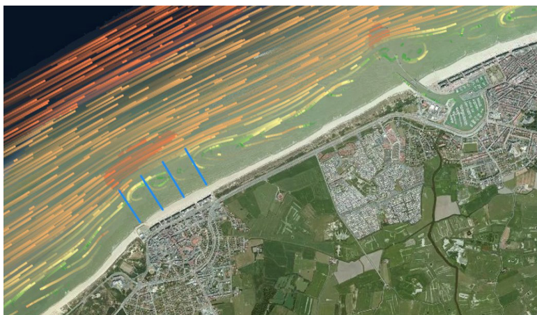
Fig. 2. Web-based dynamic visualization of XBeach hydrodynamic simulations.
