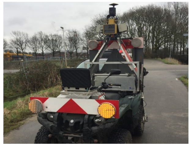
Fig. 2. 3D Laser Scanning vehicle for the inspections at the Amsterdam-Rhine Canal (Lievens 2018).
