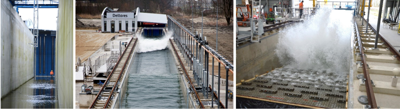
Fig. 2. Delta Flume of Deltares (left: wave board; middle: breaking wave; right: wave attack on Afsluitdijk).
