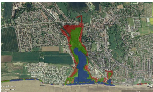
Fig 3. Range of simulated flood extents at Hornsea. Sim 0 (green), Sim 1 (blue) and Sim 6 (red) – see table 1.
