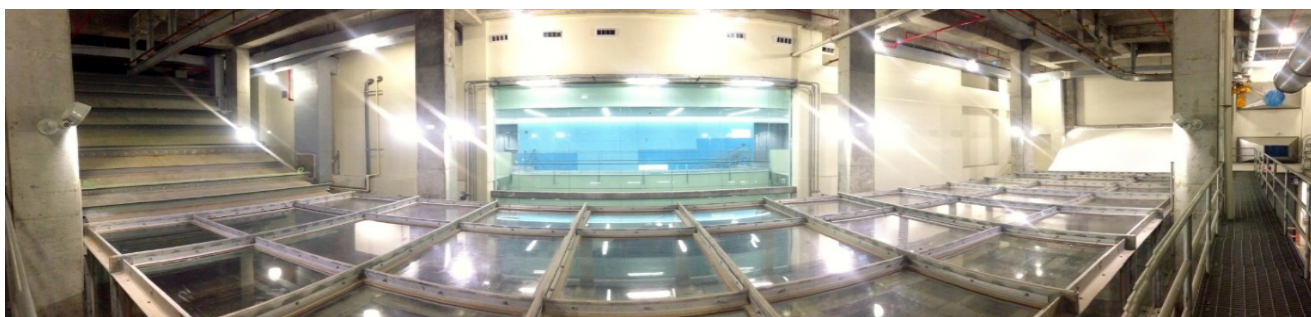
Fig. 1. Panoramic photo of the SUSTAIN tank which has dimensions 21m.-L × 6m.-W × 2m.- H.
