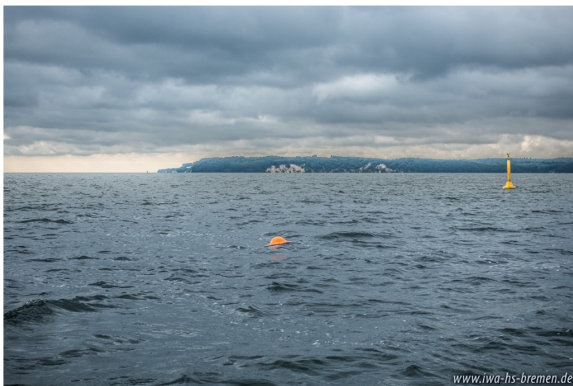
Fig. 12. Wave measurements with miniature wave buoy in the Prorer Wiek, Island of Rügen, Germany.
