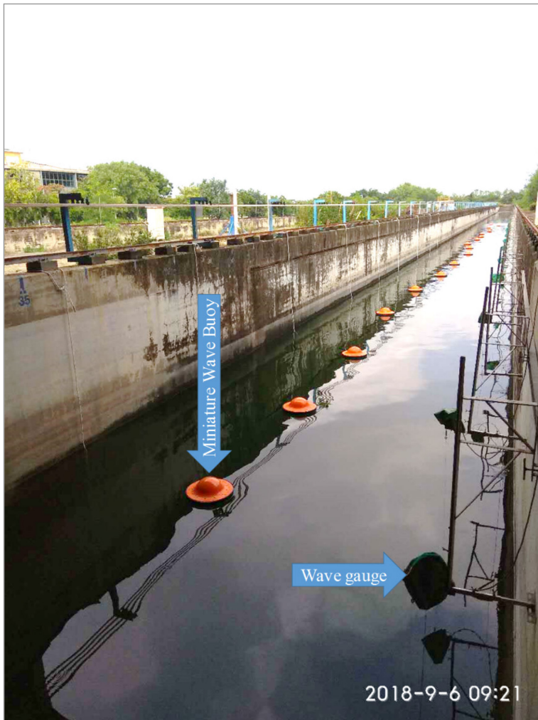
Fig. 4. Calibration testing of the miniature wave buoy in the Super Wave Flume of Tainan Hydraulics Laboratory.
