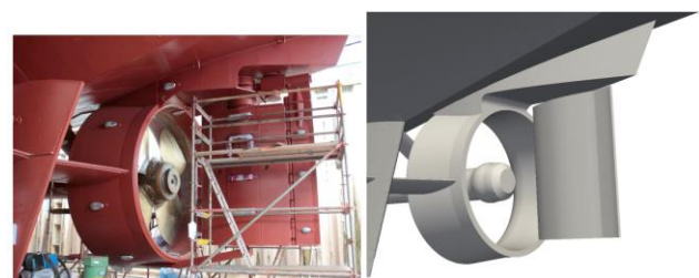
Figure 3. 3D laser scanned data of the hull and the appendages served for CFD-Simulations (Photo/Graphic: Technical University Berlin)
