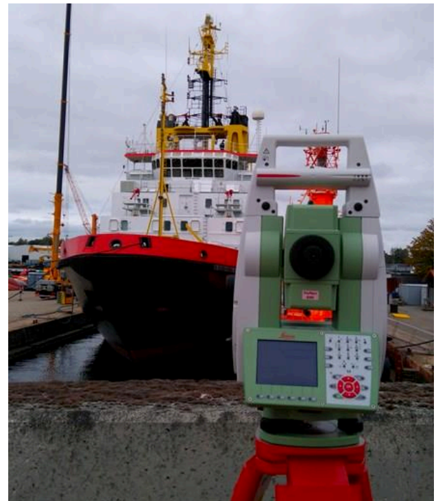
Figure 4. Determination of the sensors offsets on board (Photo: BAW)
