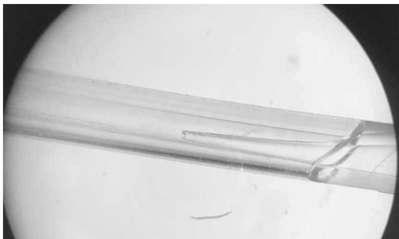
Figure 13. Simple chip with inner and outer channel used in first optimisation step, imaged under light microscope
