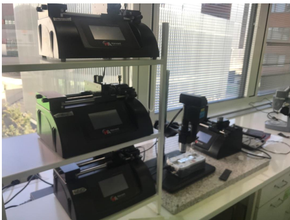
Figure 14. Setup used for optimisation and synthesis, consisted of different syringe pumps and high speed camera microscope
