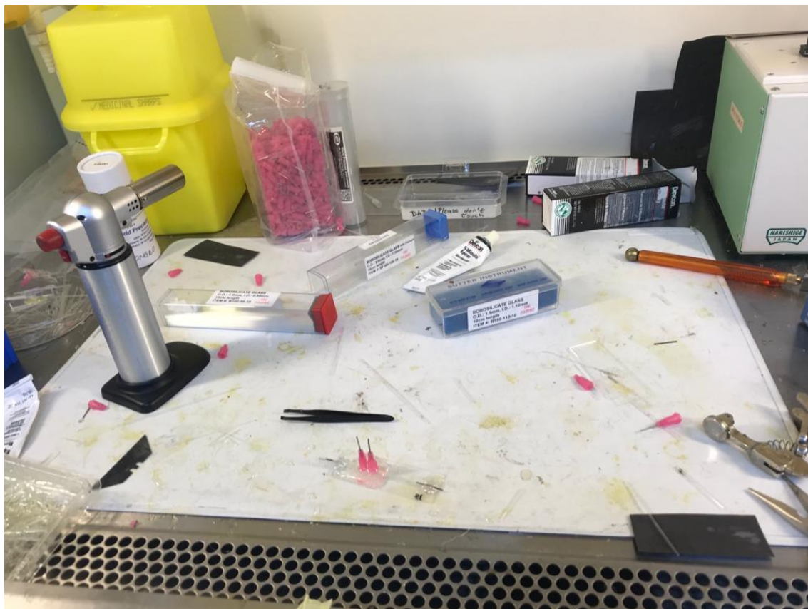
Figure 10. Small workplace under the hood that represents space exclusively intended for chip construction containing all the tools necessary as well as magnetic puller and waste
