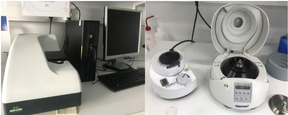
Figure 17. On the left picture there is DLS reader and vortexer and centrifuge on the right
