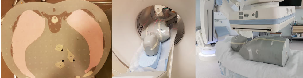
Figure 10. Example images of RPL dosimeter positioning inside the ATOM anthropomorphic phantom (left), phantom positioning on GE Discovery PET / CT table (middle) and phantom positioning on Siemens Artis Zeego table (right).
