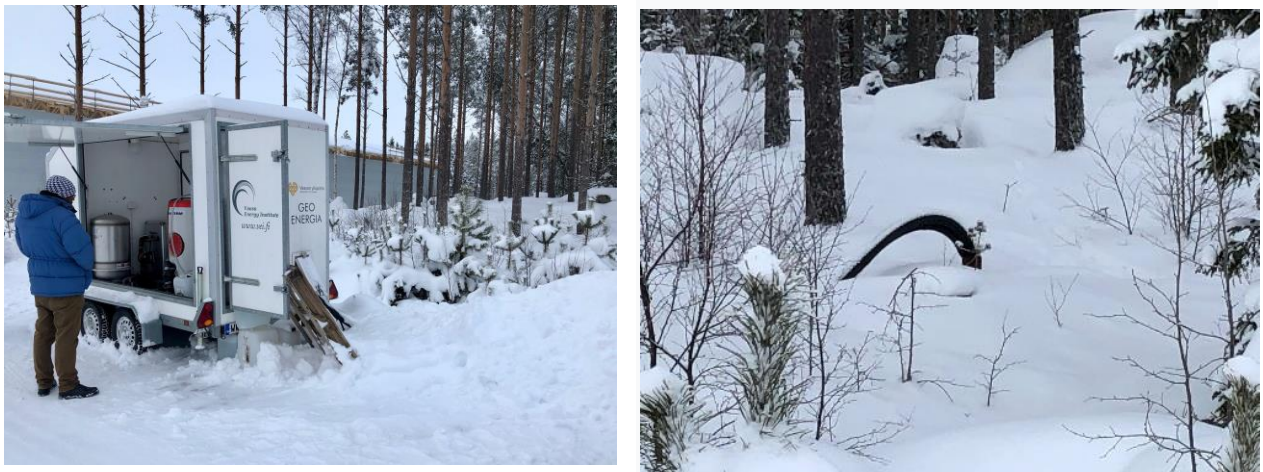
Figure 1. TRT trailer is shown in the left-hand figure. The right-hand figure shows the environment around the borehole. About 15 m long pipes go to the borehole as shown in middle of the figure.
