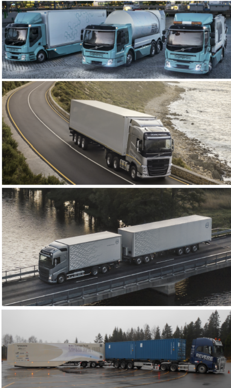
Figure 3.1: Different vehicle sizes included in the vehicle-infrastructure design. From top to bottom, they are rigid truck, tractor-semitrailer, Nordic combination, and A-double (Courtesy of Volvo Trucks).
