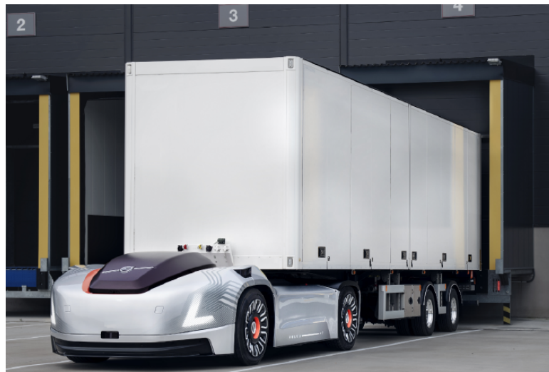
Figure 3.6: A battery electric ADS-DV (Volvo Group Vera concept, courtesy of Volvo Trucks).
