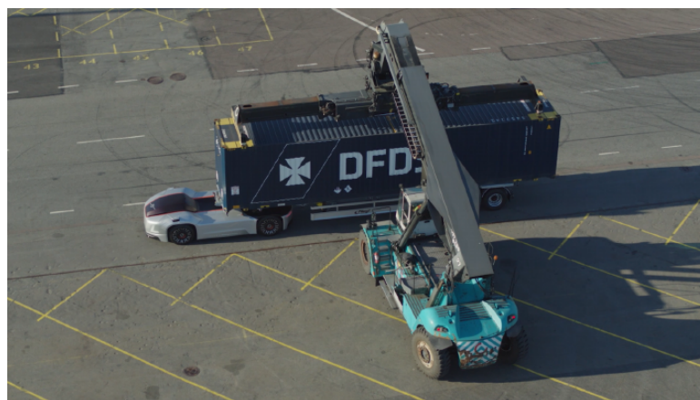
Figure 3.7: The battery electric ADS-DV unloading by a straddle carrier (courtesy of Volvo Trucks).
