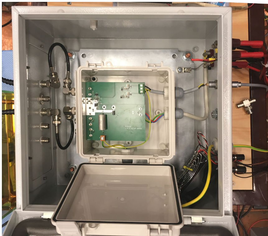
Figure 3.12 Housing of the reference impedance.
