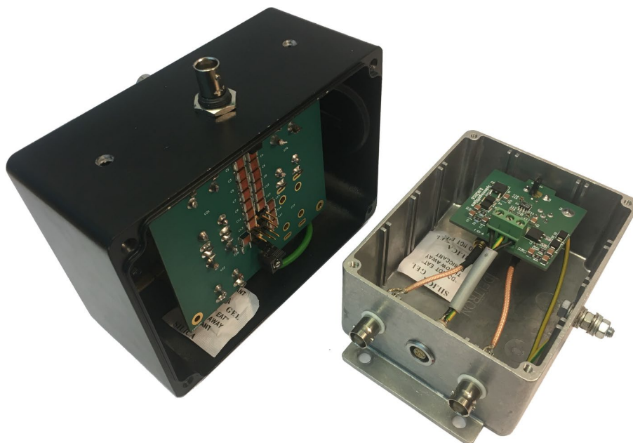
Figure 3.19: Left: the low voltage arm of the voltage divider, the air capacitors are mounted far side of the PCB. Right: The buffering amplifiers.
