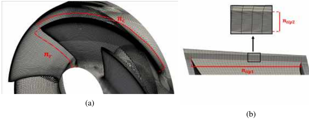
Figure 3.8: Mesh topology in the rotor region of the pump, a) surface mesh on the suction side of the rotor blade, b) mesh in the tip gap region.
