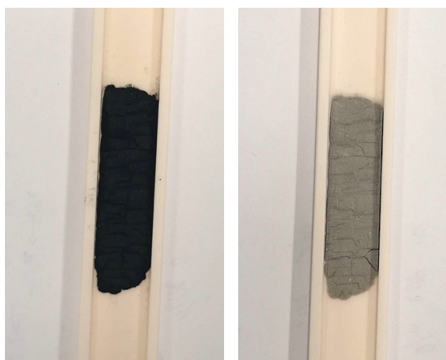
Figure 8. Metallic tellurium precursor before (left) and after (right) Experiment 5.
