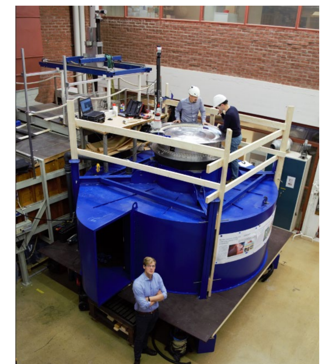
Figure 5: Schematics of Chalmers low-speed 2.5 stage heat management compressor facility. The compressor facility is currently under construction at Chalmers University of Technology, Laboratory of Fluid and Thermal Sciences. It is designed to achieve an accurate low-speed representation of a state-of-the-art low-pressure compressor designed for a future geared turbofan engine. The facility and compressor are designed to accommodate for a diversity of instrumentation and ease of access. The compressor stages can be accessed at 28 locations, six of which have traverse capabilities of a full span 18-degree sector, to be used at the rotor-stator interfaces. The traverses can be replaced with windows for optical access when performing Particle Image Velocimetry (PIV) or flow visualization within the compressor. At the rotor outlet-guide-vane interface, four independent traverse systems provide a 360-degree access for more detailed studies. The open pressure recovery at the exit of the intermediate compressor duct allows for full volume traverse access by a robot arm
