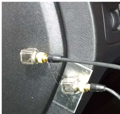
Figure 9: Two triaxial piezoelectric accelerometers placed on the cockpit left cover to measure the relative motion between the two parts.
