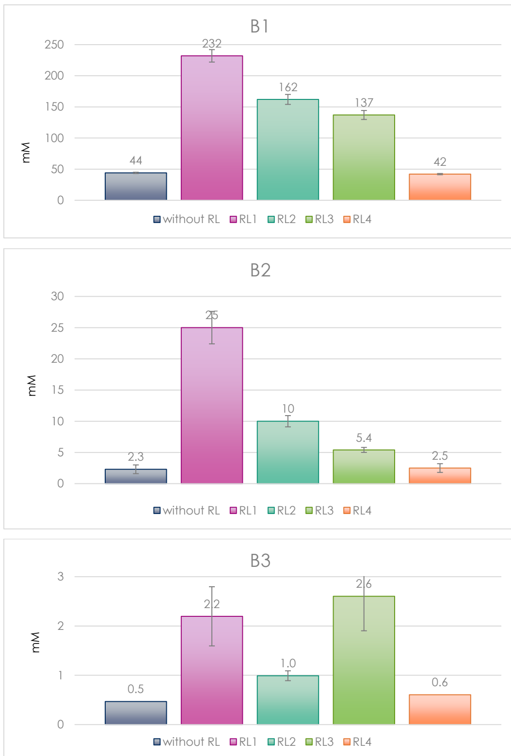
Figure 30: Ion chromatographic analysis data of the gas product (HF). B1 is the solution from the first washing bottle, B2 is the solution from the second washing bottle and B3 is the solution from the last washing bottle in the system.
