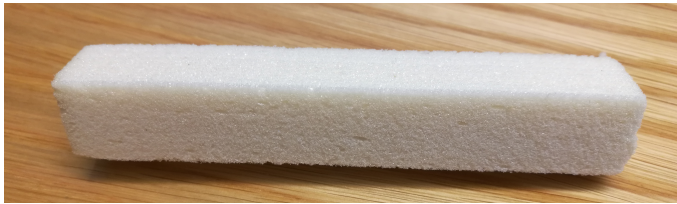
Figure 3.1: Rectangular PUR foam sample with dimensions 114 x 19 x 18 mm.
