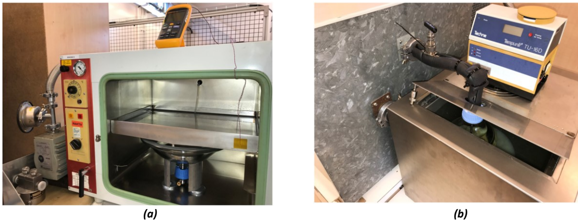
Figure 3-9. Dry oil preparation setup; A heating and vacuum chamber equipped inside with a steel tray for drying and collecting the dried oil (a), Regulated hot water bath feeding the hot oil through a needle valve into a heating and vacuum chamber (b)
