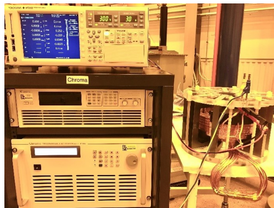
Figure 6-10. Windings loss measurement setup on prototype MFT
