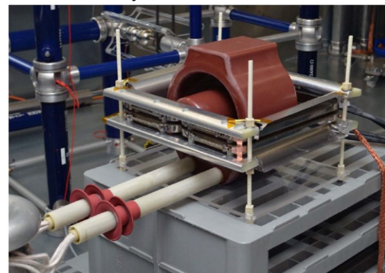
240 kVA, 0.6/0.9 kV, 10 kHz Gradinger et al. (ABB), 2017 [10] Claimed HV insulation to ground 50 kV DC PD free AC 50 Hz 35 kV
