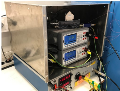
Figure 3-7. Conductivity measurement setup inside a noise suppression cage
