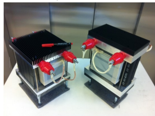
50 kW, 1/3 kV, 5 kHz Bahmani, Kharezy (Chalmers), 2014 [4] [8] Claimed HV insulation to ground 3 kV DC No information about PD test
