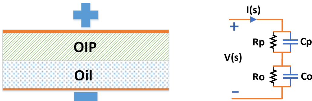
Figure 2-14. The equivalent circuit diagram of a two-layer insulation system
