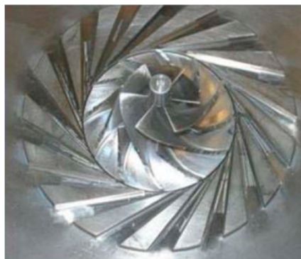
Figure 2. Solid model of the Sandia SCO 2 compressor.
