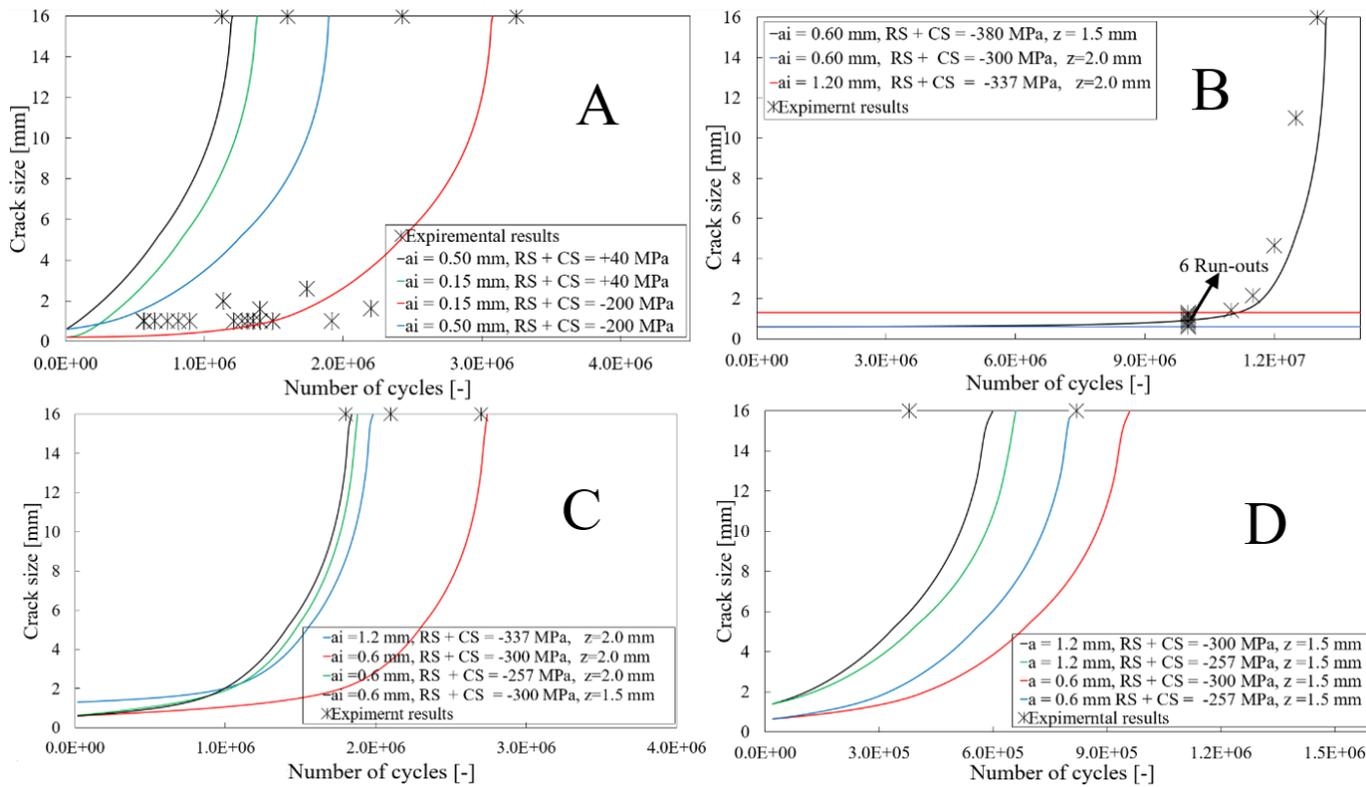
Figure 29: A: Crack propagation curves for as-welded specimen under  $\Delta\sigma = 150$  MPa
