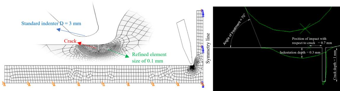
Figure 21: Elasto-plastic finite element model of cracked HFMI- Figure 22: Default values for finite element analysis
