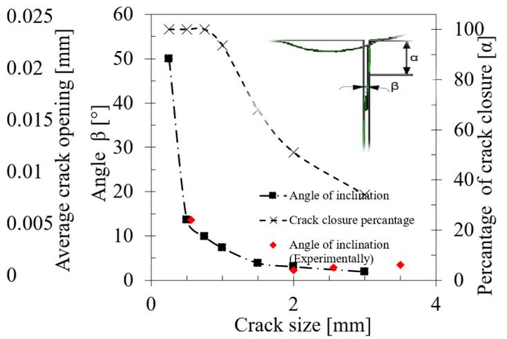
Figure 23: The dependency of contact stress and crack opening on the crack size - Figure 24: The dependency of crack inclination and crack opening on the crack size
