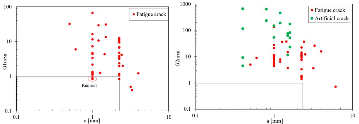
Figure 4: Gain factor  $G_1$  against depth of fatigue crack repaired by HFMI-treatment for Group 1.2
