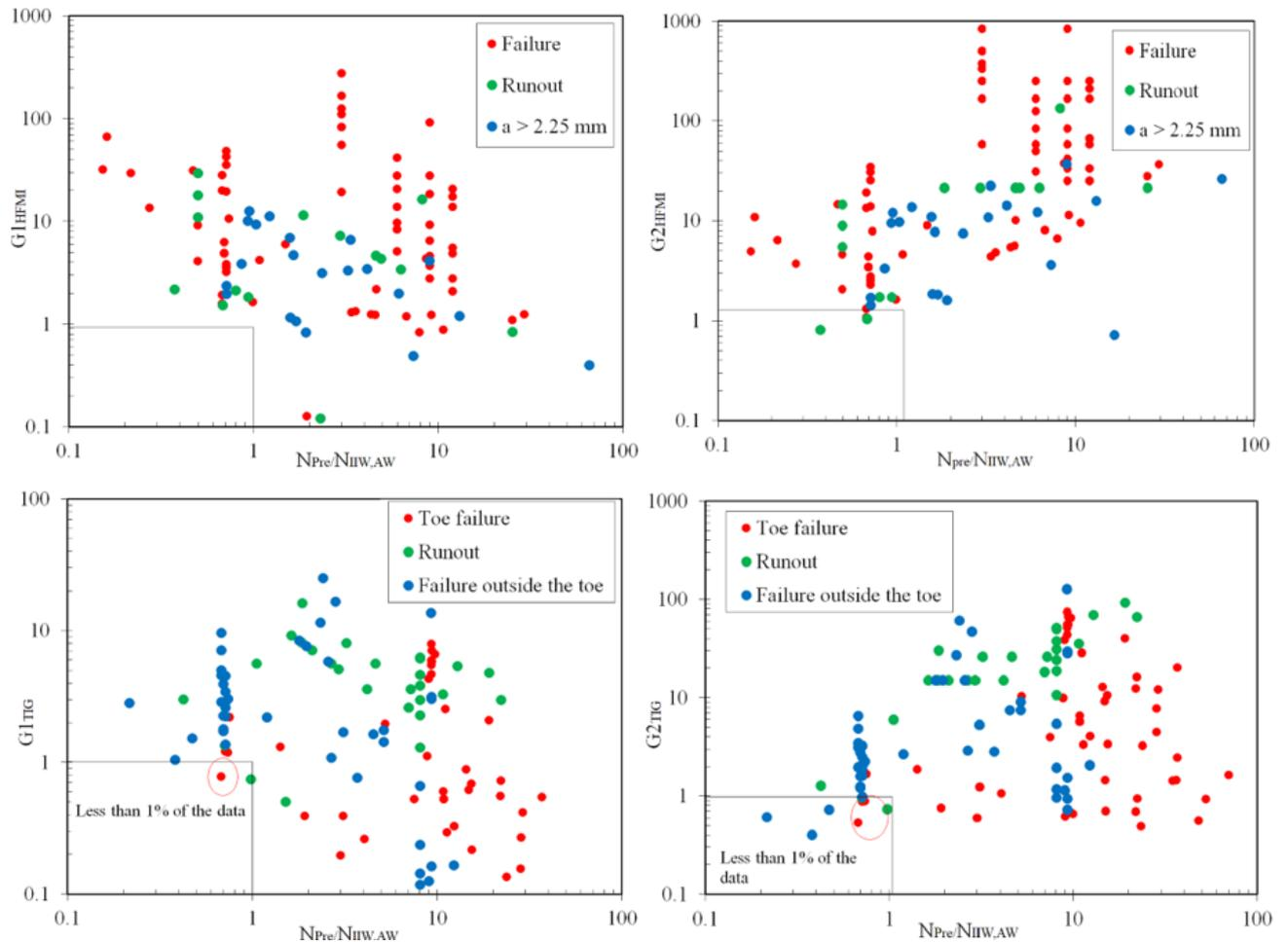
Figure 8: Gain factors against the prefatigued life before HFMI-treatment & TIG-remelting normalized to the characteristic as-welded life from IIW recommendations
