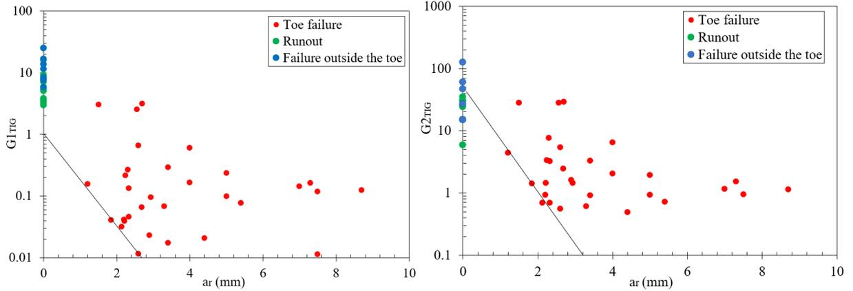
Figure 6: Gain factor  $G1$  against the prefatigued life before TIG-treatment normalised to the characteristic as-welded life for Groups 3.1 & 3.2
