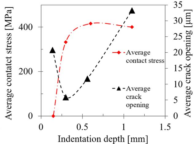
Figure 27: The indentation depth effect on cracks
