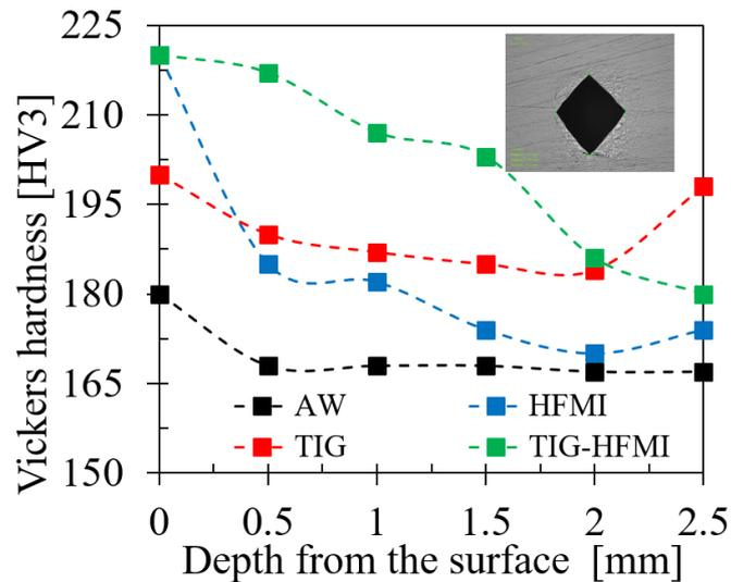
Figure 17: Vicker's hardness distribution below the weld toe
