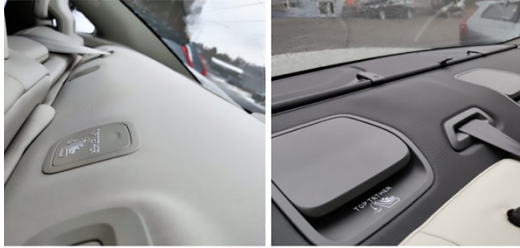
Fig. 1. (a) Current design solution for the top tether in the Volvo S90; (b) Current design solution for the top tether in the Volvo S60.
