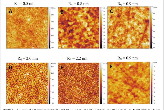
FIGURE 6 |  $\times$  5  $\mu$ M  $\times$  5  $\mu$ M AFM images of (A) TQ1A:PC<sub>61</sub>BM, (B) TQ1-50A:PC<sub>61</sub>BM, (C) TQ1-20A:PC<sub>61</sub>BM, (D) TQ1P4:PC<sub>61</sub>BM, (E) TQ1-50P4:PC<sub>61</sub>BM, and (F) TQ1-20P4:PC<sub>61</sub>BM films processed from the same solution as device fabrication.
