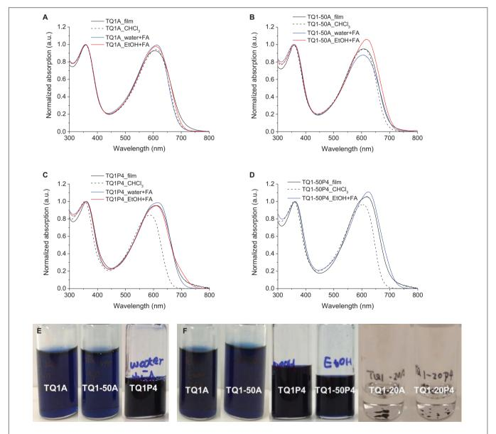
FIGURE 1 | Normalized UV-vis absorption spectra of (A) TQ1A, (B) TQ1-50A, (C) TQ1P4, and (D) TQ1-50P4 in different solvents and in the solid state. Photographs of (E) polymer in water + 3% FA solution, (F) polymer in EtOH + 3% FA solution.
