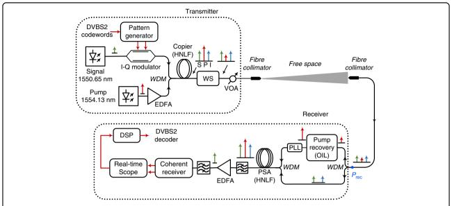
**Fig. 4 Detailed experimental set up of the free-space communication system with a PSA pre-amplified receiver.** EDFA erbium-doped fibre amplifier, HNLF highly nonlinear fibre, OIL optical injection locking, WS wave shaper, VOA variable attenuator, WDM wavelength division multiplexer coupler, DVBS2 digital video broadcasting standard 2 code, PSA phase-sensitive amplifier; the electrical paths are indicated by red lines; the optical paths are indicated by black lines
