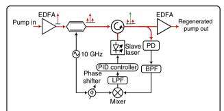
**Fig. 5 Experimental setup of optical injection locking with the PLL.** PD photodetector, PID proportional integrator differentiator, BPF bandpass filter, LPF low-pass filter, EDFA erbium-doped fibre amplifier; the red lines indicate the electrical paths, and the black lines indicate the optical paths
