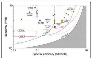
Fig. 3 Sensitivity (photon-per-information-bit, PPB) versus spectral efficiency (bits/s/Hz) with different implementations.
