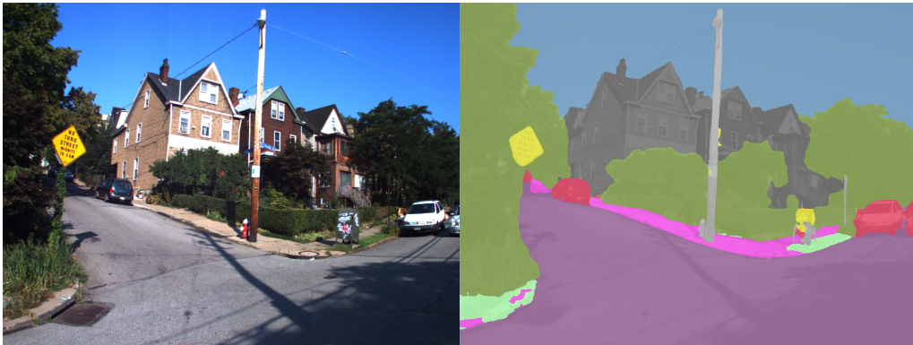
Figure 3.6: (Left) Example of an image from a road environment and its semantic segmentation. (Right) The same image colorized according to class by a semantic segmentation algorithm.
