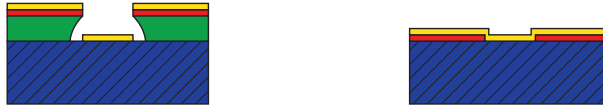
Figure 6.2: (left) With the presence of the undercut, the metal layer (yellow) is not continuous and allows the remover to access the resist. (right) Without the undercut and lift-off layer, the metal forms a continuous layer on top and remover can't access the resist.
