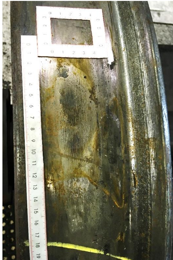
Figure 6: Wheel with a long wheel flat
