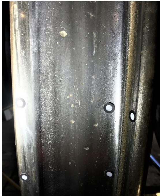
Figure 5: Wheel with indentations on the tread. The black and white dots were used as markings during the 3D scanning activities of Paper A
