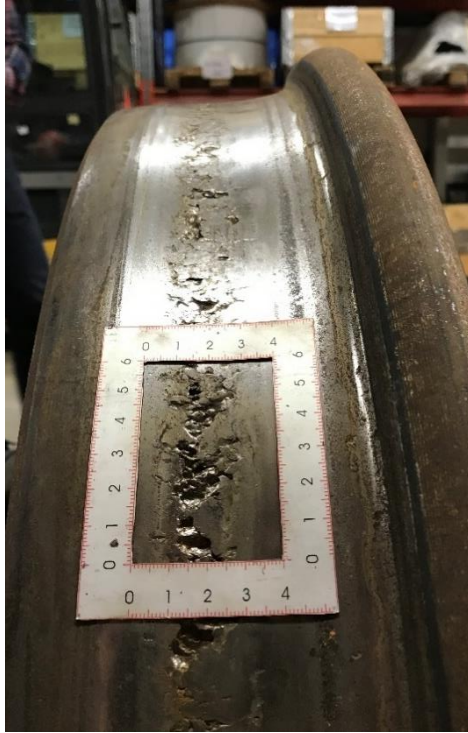
Figure 4: Wheel from a passenger train with severe RCF damage
