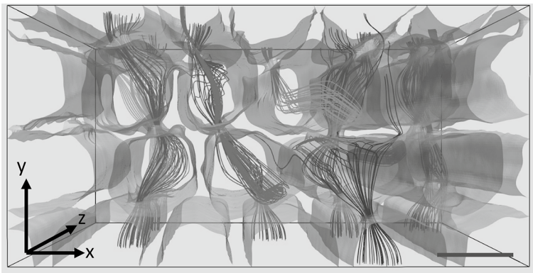
Fig. 10 Simulation box surrounding the surface of Case 4 with streamlines generated from a point source following the flux field. The radial and tangential directions are y and x , respectively, and z is longitudinal. The scale bar in the lower right corner is 25\ \mu\text{m} . The color of the streamlines indicates different pathways from tracheid to tracheid through the bordered pits
