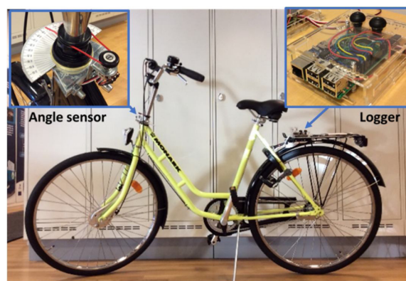
Fig. 1. Instrumented bicycle: a classic urban 3-speed bicycle with a step-through frame, a rear coaster brake, and a drum brake on the front wheel; the instrumentation, powered by a power bank, comprises an angle sensor, an inertial measurement unit, a speed sensor, and a logger.
