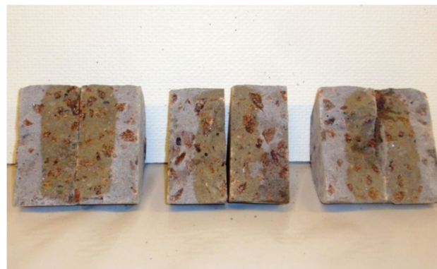
Figure 5. Test specimens for the Rapid Chloride Migration test after being sprayed with silver nitrate solution.
