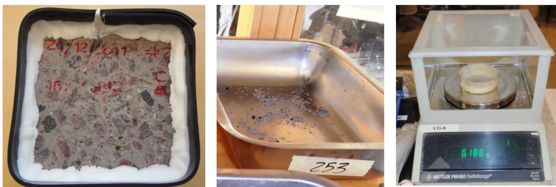
Figure 8. Left: Example of specimen after 112 freeze/thaw cycles (specimen of Mix 2%-25% GGBS, 4.5% Air, k = 0.6 ); Center: Scaled-off material collected on a steel vessel; Right: Determination of the mass of scaled material.
