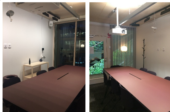
Fig. 1. Inside the test offices: office 3104 to the left and 4104 to the right. Aldehyde and TVOC samplers are fastened on the disks hanging from the spot-light rails below the ceilings.
