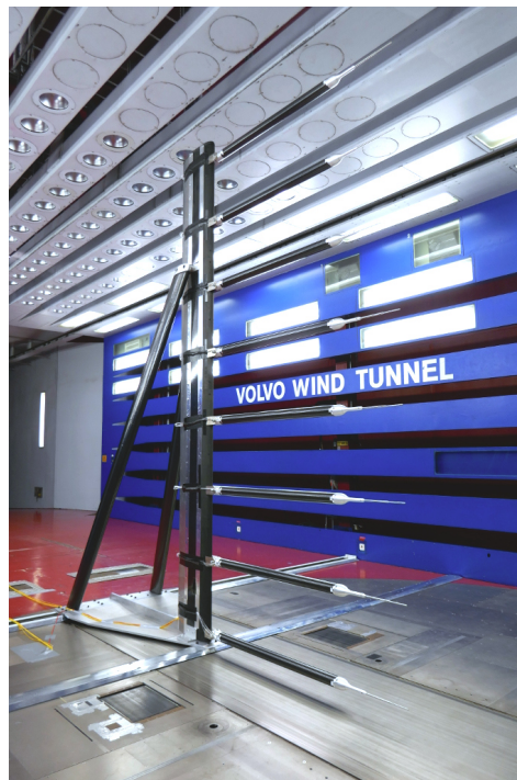
Figure 5. The Volvo PVT flow measurement rig (FMR).
