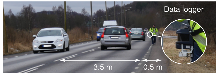
(a) Field test data collection to record pedestrian-overtaking maneuvers.
