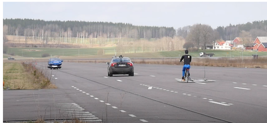
(b) Test-track data collection to record cyclist-overtaking maneuvers.
